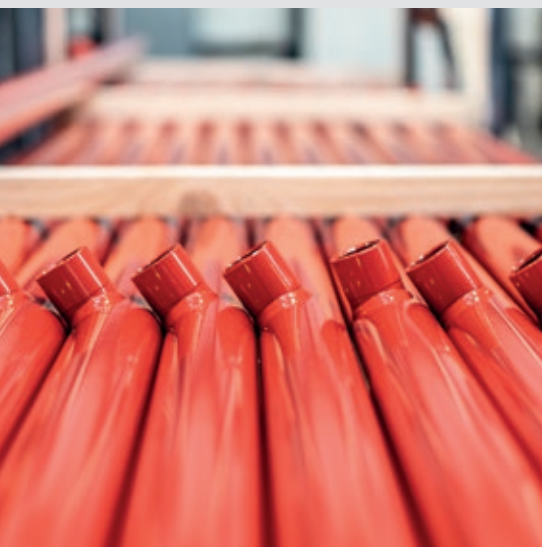
Pipes with welded on sleeves for sprinkler heads
